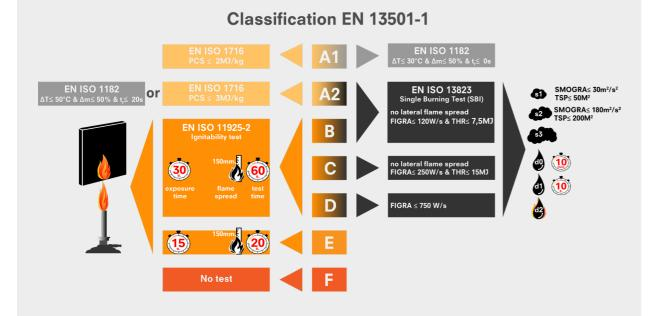
There are some particular cases, for example A1 coated building material (e.g. painted solid metals) requires an SBI test in order to check the fire behaviour of the painted surface.
