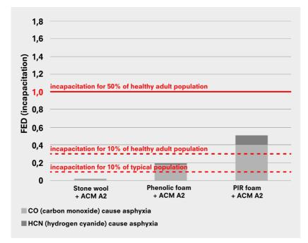
Contribution of CO, HCN, CO, and lack of O, to lethality (ISO 13344) at 30 minutes for gases entering a 50m<sup>3</sup> room from cladding through 100mm vent:
