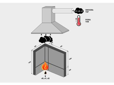
The classification parameters of the SBI test are fire growth rate index (FIGRA), lateral flame spread (LFS), and total heat release (THR600s). Additional classification parameters are defined for smoke production as smoke growth rate index (SMOGRA) and total smoke production (TSP600s), and for flaming droplets and particles according to their occurrence during the first 600 seconds of the test.
