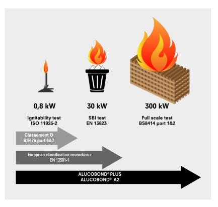
ALUCOBOND® completed full scale tests in accordance with BS 8414 and then in getting an assessment in accordance with BR 135:
